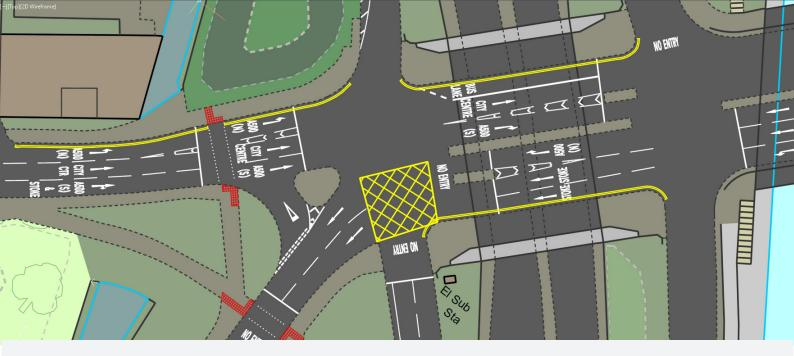
Road users rely on a range of cues to help them navigate their trips safely and efficiently. Among the most essential types of markings include lane lines, directional arrows, pedestrian crossings, bus and cycle lanes. The design and placement of these elements are carefully considered
